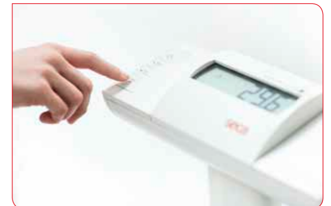
With the seca 360° wireless technology and the press of a key, the seca 703 can send measurements to an optional seca 360° wireless printer or seca software on the PC.
